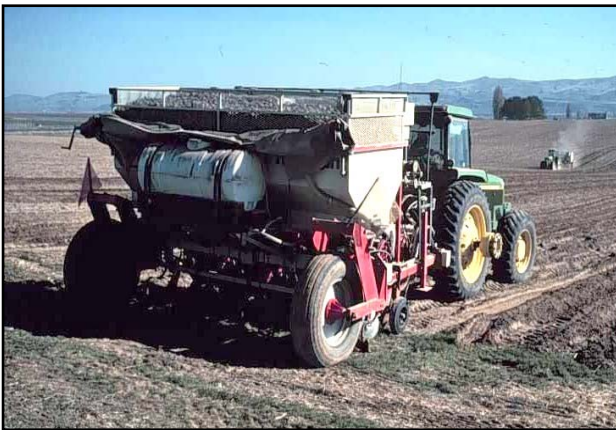
Figure 12a. Semi-mounted potato planters are used widely. Potato planters come in two-, four-, six-, or eight-row units. Picker-arm and cup-type planters are the most popular (left). (M. Pavek)
