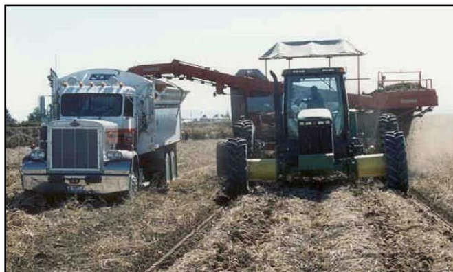
Figure 22. Potatoes are harvested with two-row or four-row harvesters. Windrowers which place two or four rows of potatoes in the center of un-dug rows increase the efficiency of harvesters. Tubers are placed in bulk-bodied trucks and transported to grading areas, storages, or processing plants.
